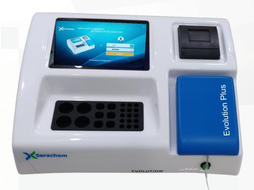
Semi - Automatic Chemistry & Coagulation Analyzer
